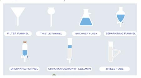
**Filter funnel** into which filter paper can be placed, and a mixture can then be poured through. The smaller *thistle funnel* is not used for filtering at all, but to add liquids into apparatus.
