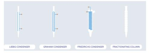
**Graham condenser** is like this but has a coiled path for the vapour to flow through and condense. Meanwhile, the *Friedrichs condenser* inverts the arrangement, having a spiral coil through which the coolant flows, with the vapour surrounding it. Other varieties of condenser are also available, though are not shown here.
