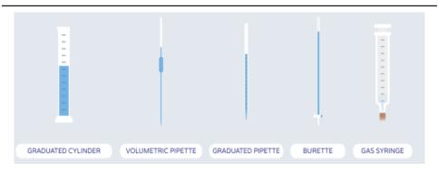
**Volumetric pipette** which can be used to measuring volumes of solutions more precisely. These come in a variety of sizes, each measuring a fixed volume of solution.
