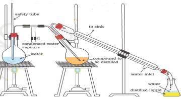
Steam distillation. Steam volatile component volatilizes, the vapours condense in the condenser and the liquid collects in conical flask.
